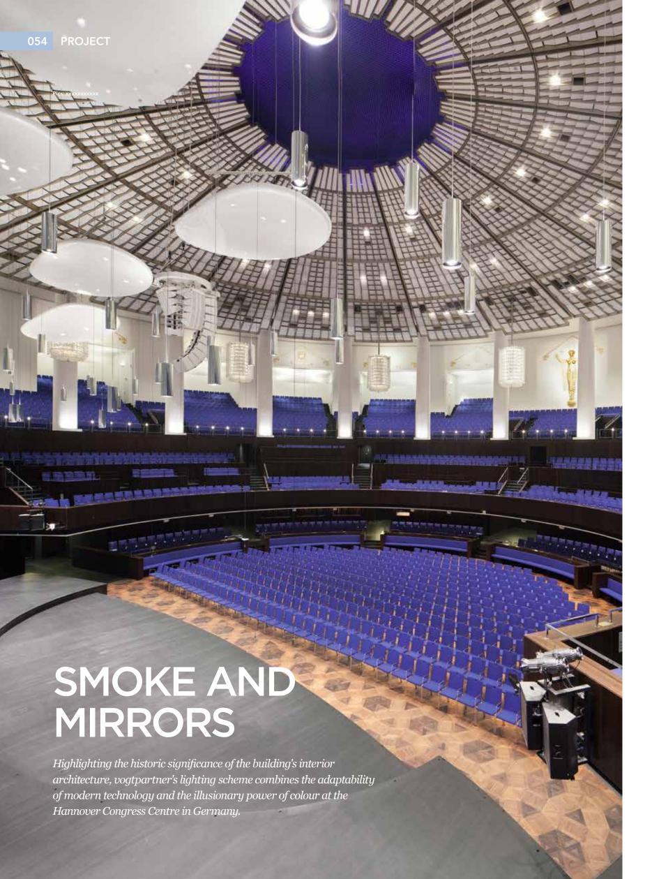
With the removal of former acoustical components above the stage area, the entire ceiling becomes more noticeable. Suspended above the stage, freely arranged custom pendant luminaires from Hagenauer evoke the image of a transparent 'light cloud'. The luminaires can be lowered or raised as a group and are dimmable. Their highly specular surface reflects surrounding colours, making them almost invisible.
